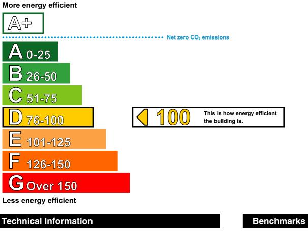
Grid Supplied Electricity Main heating fuel: Building environment: Air Conditioning 126 Total useful floor area (m<sup>2</sup>): Building complexity (NOS level): 3 Building emission rate (kgCO<sub>2</sub>/m<sup>2</sup>): 121.91
